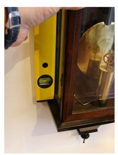
Adjust the case position on the wall so that it is similar to that shown in the photo using the spirit level. The case isn't square after all these years, so the angle on my wall that looked best is when the spirit level was placed on the back left section as shown. If you prefer a different angle that's fine, but you are likely to have to make an adjustment. The clock is set up in beat for the angle shown.
