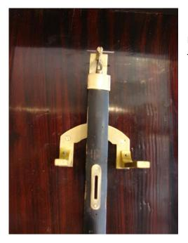
Hang the pendulum on the suspension spring fixed to the top of the mounting bracket.
