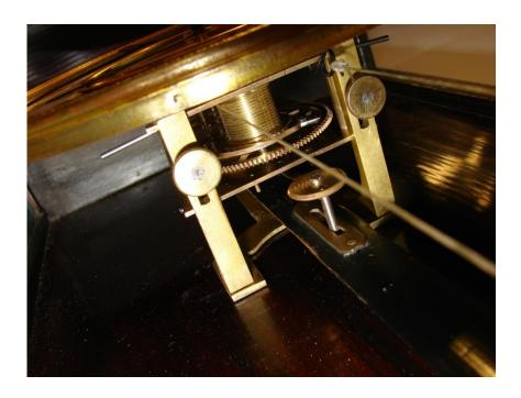
Wind up half a turn only using the key provided. Turn the key clockwise.
