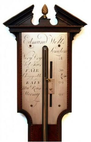
A George III mahogany barometer with well-engraved silvered dial signed Edmund Wells, London. The break-arch pediment has a pineapple brass finial, over the engraved silvered brass register plate, signed by the maker and bearing a manually-operated vernier.
