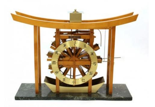
This is a 1970s version of the ancient waterwheel clock, a form of clepsydra largely based on a design which has been in existence in East Asia for around 2000 years.
