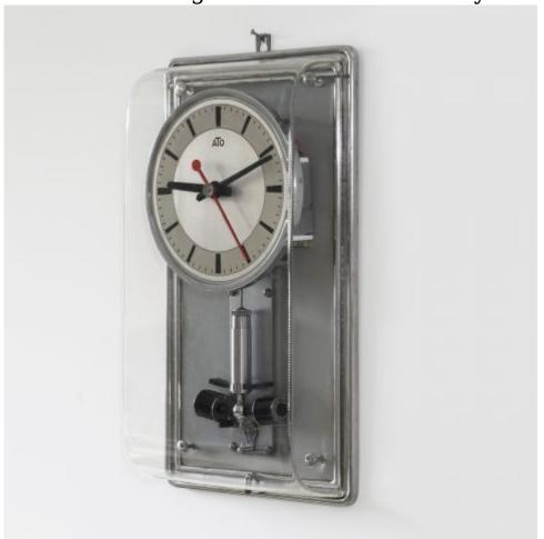
A French electric industrial vintage wall clock made by ATO, dating from the 1950s. This is a very early example of the use of transistors in clocks.
