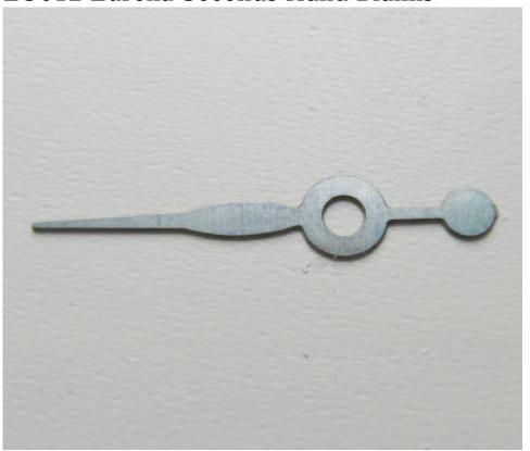
These hands are cut by Laser in Stainless Steel from a pattern taken from an original. The hand is 14mm from tip to centre of mounting hole and 21mm overall.
