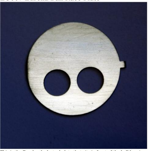
This is the Eureka clock steel plate that sits in front of the ball bearings, as shown in Figure 34, page 47 of *The Eureka Clock*, by Dr. Alan Shenton. It is made using 0.25mm spring steel.
