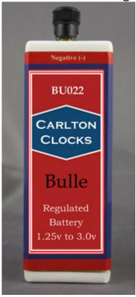
This battery is a direct replacement for the original 1.5v Bulle battery No23 which is no longer available. The size (125mm x 40mm x 40mm) is slightly shorter than the No23 and is designed to fit the column of the tall "A" movement clocks. It will also fit many other Bulle clocks but NOT a clockette\* (height includes terminals).
