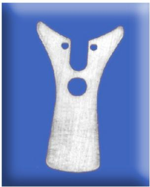
These forks have been cut in 0.20mm Carbon Spring Steel from a pattern taken from an original. They are made to fit the Tall Bulle movement and will need to be finished with the Silver contact and Fibre insulator.
