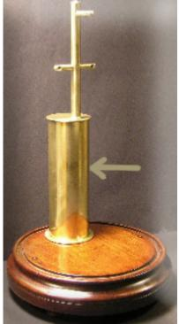
If you have ever had a Bulle clock which has had leaky batteries then you will probably be familiar with the state of the column shown at the right hand side of the first photo. A gaping hole burnt through by battery acid.
