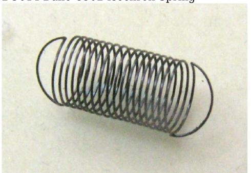
These Isochron springs are made to the original design but are made from 0.15mm C902 steel instead of Invar. 18 coils of 4mm, 2 half end coils at right angles. They are the only springs that are consistent with the compositional characteristics of the original Bulle spring as shown in the laboratory test conducted over 2004 / 2005. The original patent specifies Invar, but this is much too soft for use as a spring. Each is supplied in a clear perspex box.
