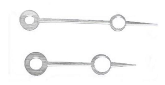
These hands are cut by Laser in 0.70mm High Carbon Spring Steel from a pattern taken from a pair of originals.
