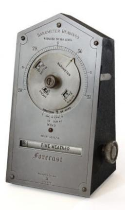
A very nice example of Negretti & Zambra's desk weather forecaster, dating from c.1920. This makes a perfect companion piece to a barometer or barograph, where the readings can be hard to interpret.
