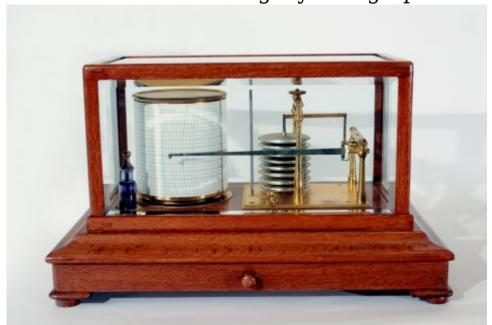
A fine example of a mid C20th, mahogany, 8-stack recording barometer by Short & Mason, first retailed by the Army & Navy Stores Limited, and numbered I.30034.
