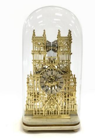
An imposing three train fusee skeleton clock by Evans of Handsworth from c.1870, based on the design of Westminster Abbey. The design is very three-dimensional, having four fretted brass frames; two contain the movement, a third supports the dial, and a fourth small frame is the entrance porch. The frames are beautifully fretted out, and carry silvered plaques for the retailer *A Everington, Nottingham*.
