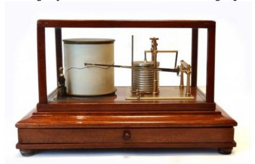
A good antique mahogany-cased barograph, with a tall vaccuum chamber, by Short & Mason. The case has a drawer for storing spare / used charts, and its original glass ink bottle recessed into the case at the left hand side near the drum.
