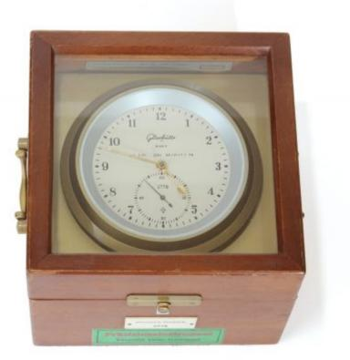
Dating from 1986, this German-made Glashütte Type 1-71 quartz marine chronometer clock is a fine quality desk clock that keeps excellent time, to within a second in a week.
