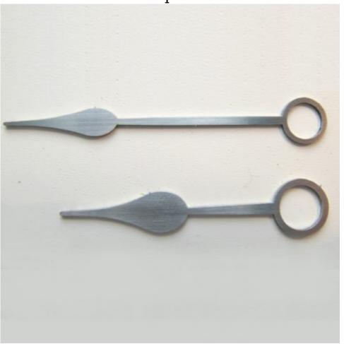
These hands are cut by Laser in 0.70mm High Carbon Spring Steel from a pattern taken from a pair of originals. The hour hand is 40mm from tip to centre of mounting hole. The minute hand is 53mm from tip to centre of mounting hole. Both will need to be polished & blued and have collets made to fit.
