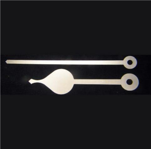
These hands are cut by Laser in 1.0mm thick aluminium from a pattern taken from a pair of originals. The minute hand is 160mm from tip to centre of mounting hole. The hour hand is 129mm from tip to centre of mounting hole. Both will need to be painted and have collets made to fit. Price includes recorded delivery within mainland UK.
