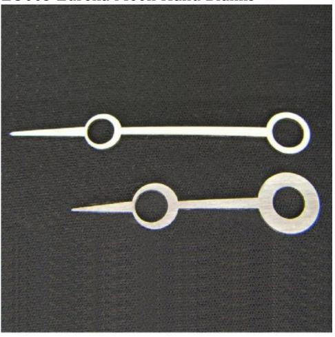
These hands are cut by Laser in 0.70mm High Carbon Spring Steel from a pattern taken from a pair of originals.
