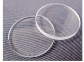
These superb hardened glass discs for the Eureka clock are 2.5mm thick and 22.0mm diameter. Many Eureka clocks are found with broken and smashed bearing glass which impairs both function and aesthetics. These smooth machined edge disc are much harder than the ground edge EU001 which they replace.
