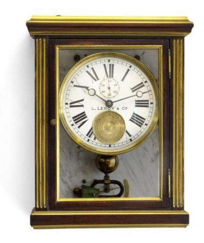
This is an interesting example of an electric regulator wall clock dating from the 1930/40s. When new, these Brillié clocks could be regulated to an accuracy of +/- 1 sec/day.
