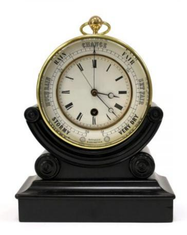
A rare 1860s Bourdon and Richard's Patent ships-style combined clock/metallic barometer. The brass drum-shaped case has been polished and lacquered. It has a suspension ring to the top, and rests on an ebonised wooden stand.
